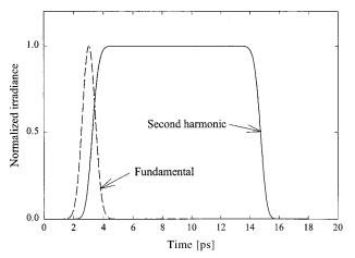
Fig. 1. Normalized irradiance of the fundamental and secondharmonic output from a 10-mm-long BBO crystal in the lowconversion regime. The input fundamental is a 1-ps (FWHM) Gaussian pulse. The second harmonic is stretched by 12 ps because of the group-velocity difference between the fundamental and the harmonic waves.
