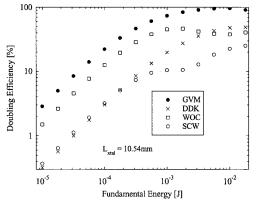
Fig. 12. Doubling efficiency versus fundamental pulse energy for a total crystal length of 10.54 mm for a single crystal with no walk-off (GVM) (filled circles), for a single crystal with walk-off (SCW) (open circles), for five WOC crystals (open squares), and for five crystals with phase-matching frequencies separated by half of the crystal acceptance bandwidth (DDK) (crosses).
