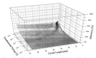
Fig. 9. Doubling efficiency versus crystal length and fundamental pulse energy for a crystal with BBO's group-velocity walk-off (SCW).
