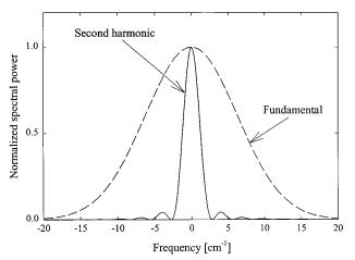
Fig. 2. Normalized spectra of the pulses of Fig. 1. The fundamental is a Gaussian of width (FWHM) 440 GHz (14.7 cm<sup>-1</sup>). The harmonic is the product of a Gaussian and a  $|\operatorname{sinc}(\Delta \omega t)|^2$  function with its first nulls at ±83 GHz (2.8 cm<sup>-1</sup>).
