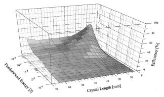
Fig. 11. Doubling efficiency versus total crystal length and fundamental pulse energy for five crystals with detunings  $\Delta \omega = -13.9, -6.94, 0, 6.94$ , and 13.9 cm<sup>-1</sup> (DDK).
