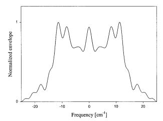
Fig. 5. Envelope function for five crystals with detunings  $\Delta \omega = -13.9, -6.94, 0, 6.94, and 13.9 \text{ cm}^{-1}$ .
