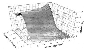
Fig. 8. Doubling efficiency versus crystal length and fundamental pulse energy for a crystal with no group-velocity walk-off (GVM).
