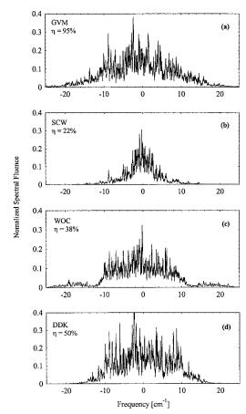
Fig. 6. High-conversion efficiency normalized harmonic spectra under the same conditions as Fig. 3 except the fundamental pulse energy is increased from 10  $\mu$ J to 10 mJ.
