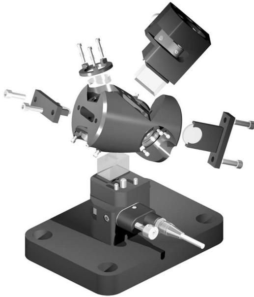
Fig. 3. Exploded solid rendering of two-crystal RISTRA cavity assembly showing cylindrical body, spring-loaded three-point mirror retainers and mirror substrates, wave plate holders, and crystal rotation assemblies. Owing to its nonplanar geometry, the RISTRA requires no cavity mirror adjustments. See text for additional details.
