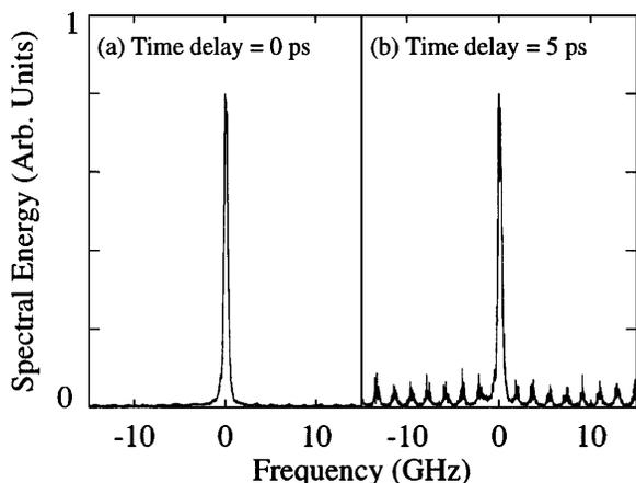
Fig. 3. Scanning Fabry-Perot étalon spectrum of 532-nm light produced by sum-frequency mixing of the signal and the idler for unseeded operation. The étalon free spectral range of  $\sim 40$  GHz is less than the unseeded OPO linewidth.
