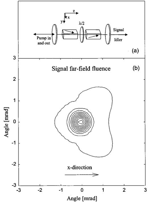
Fig. 15. (b) Far-field signal fluence for the cavity of (a) and operating parameters of Table 1.
