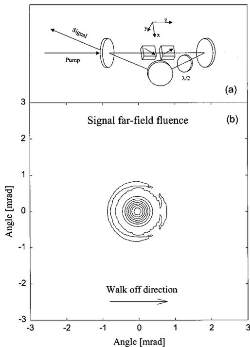
Fig. 10. (b) Far-field signal fluence for the cavity of (a) and the operating parameters of Table 1.
