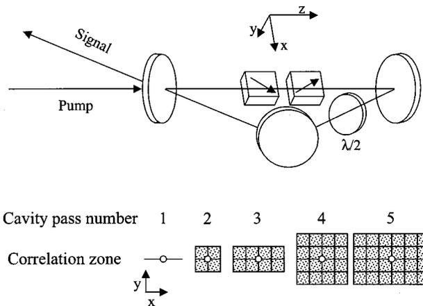
Fig. 9. Cavity design for two walk-off-compensating crystals oriented with walk-off in a plane rotated 45° relative to the plane of the cavity. The expanding zones of correlation for the signal wave after successive crystal passes are shown at the bottom, demonstrating their symmetric growth.
