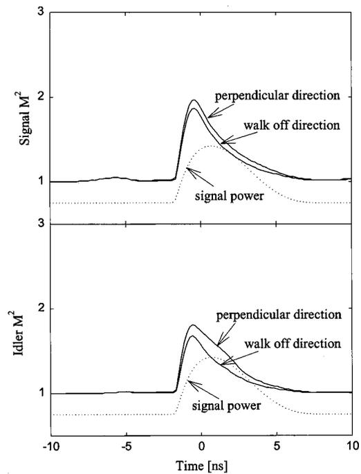
Fig. 16. (a) Signal and (b) idler beam quality as a function of time for the OPO of Fig. 15(a). Dotted curves, signal power in arbitrary units, shown for reference.
