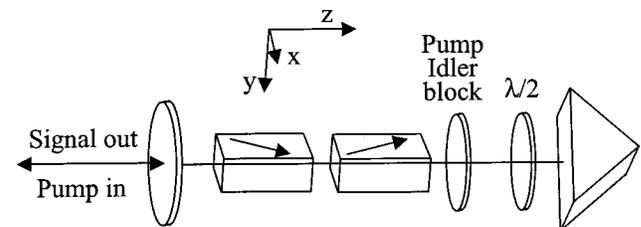
Fig. 12. Standing-wave equivalent of the ring OPO diagrammed in Fig. 10(a).
