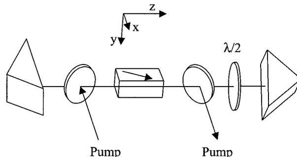
Fig. 7. Image-rotating OPO cavity design based on rotated roof prisms. The wave plate rotates the signal polarization by 45°. The pump can be coupled by use of intracavity mirrors that pass the signal and reflect the pump. Signal output coupling could be accomplished through frustrated reflection at one of the prisms, or a prism could be replaced with partially reflecting mirrors in a rooftop configuration.
