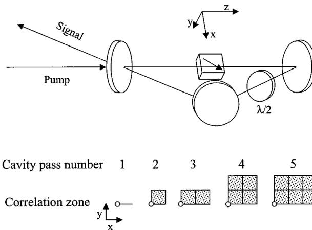
Fig. 8. Cavity design for a crystal oriented for walk-off in a plane rotated 45° relative to the plane of the cavity. The expanding zones of correlation for the signal wave after successive crystal passes are shown at the bottom, demonstrating their asymmetric growth with respect to the origin.
