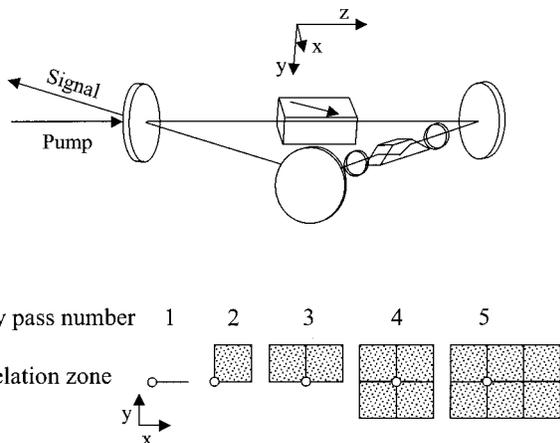
Fig. 4. Image-rotating OPO cavity design based on a dove prism image rotator. Half-wave plates before and after the dove prism rotate the signal polarization by  $45^\circ$ . The expanding zones of correlation for the signal wave after successive crystal passes are shown at the bottom.
