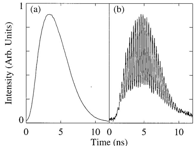
FIG. 3. OPO signal pulses measured with a 3.2 GHz bandwidth detection system: (a) undisturbed pulse and (b) after passing through an absorption cell filled with room temperature rubidium vapor. The seed wavelength was tuned to the Rb  $5S_{1/2} \rightarrow 5P_{3/2}$  resonance at 780 nm for this measurement.
