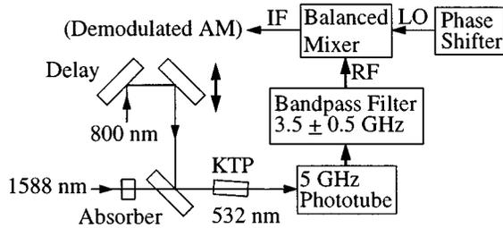
FIG. 1. Diagram of the FM-seeded OPO and AM detection apparatus. (VCO) voltage-controlled oscillator.
