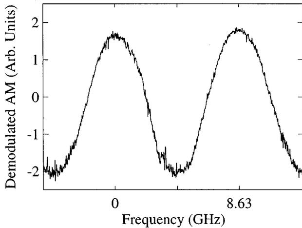
FIG. 4. Spectrum of demodulated AM normalized to the 532 nm signal-idler sum-frequency-mixed pulse energy. The spectrum is generated by placing an 8.63 GHz free-spectral-range uncoated optical flat in the 1588 nm idler beam and scanning the 800 nm FM light that seeds the OPO.
