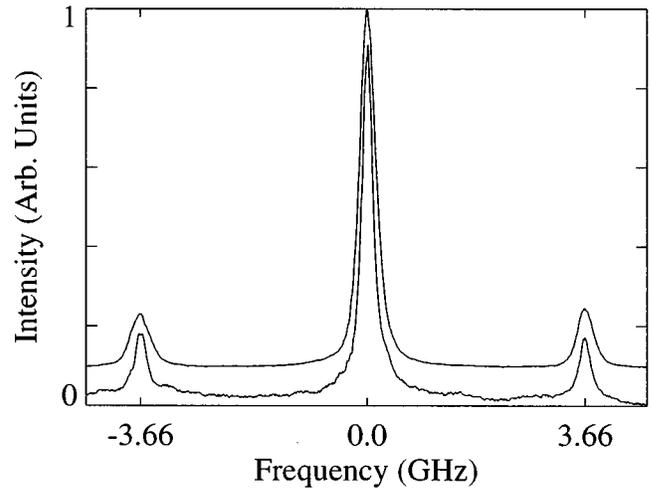
FIG. 2. Scanning Fabry-Perot étalon spectra of the FM seed (lower) and OPO signal (upper). Spectra are offset for clarity.
